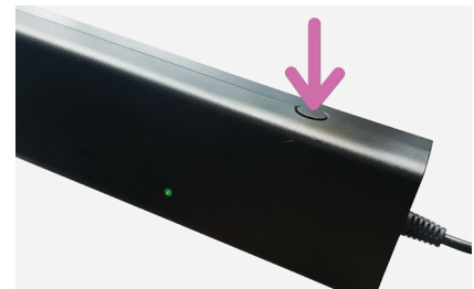
Learn button on the power supply unit.
