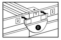
Use threaded holes on elevate kit to attach and secure 6 legs. To return base to it's original height. REMOVE ONE SECTION OF THE 3-IN-1 LEG.
