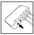
Double click the PAIR button on the control box (light will turn blue during the pairing process).
