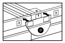
Use threaded holes on elevate kit to attach and secure 6 legs. To return base to it's original height. **REMOVE ONE**
